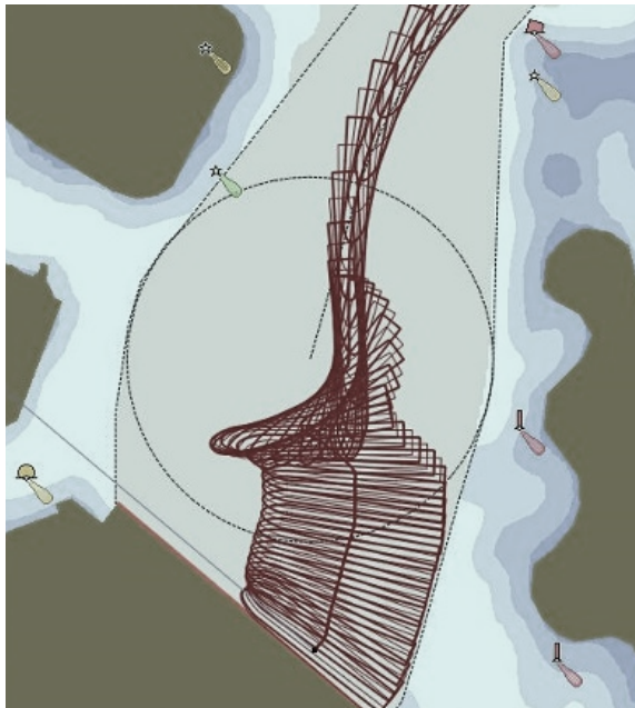
Figure 3 Simflex4 vessel navigation in conceptual extents of the Port Victoria basin. Image represents a vessel (dark red outline) entering the port under calm conditions with tug assistance.
